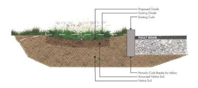
above: Good Approach. Simple bioswale is constructed behind the existing Folly Road curb with amended native soil and plantings.
