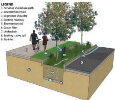
above: Town bioretention "typical" – encourages infiltration in areas of well draining soils
