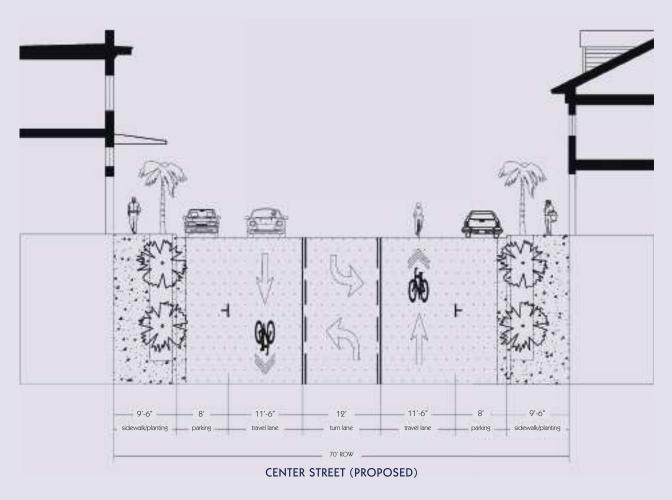
On Center Street (Folly Beach), the street is proposed to be reduced to three lanes with a center turning lane and onstreet parking on either side. This roadway reconfiguration has been proposed by others (Stantec). In addition to the lane reallocation, the proposed section above recommends shared lane markings be added to the travel lanes. Onstreet parking could be permeable pavement material.
